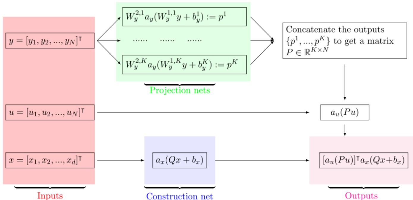
BelNet is a generalization of DeepONet: it projects  $u$  into the space spanned by a trainable basis  $p$ . FNO is a special case of BelNet.
