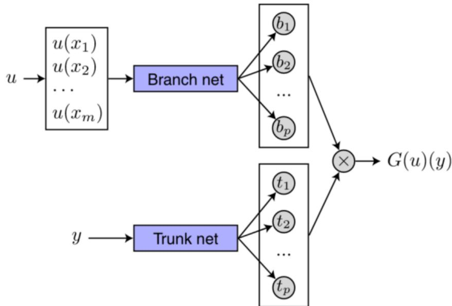
The **trunk** learns *basis functions* and the **branch** corresponding *coefficients*.
